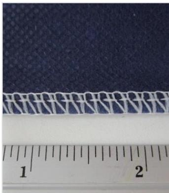
Figure 2. Stronger 4-thread overlapped seam
