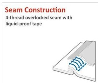
Figure 4. Overlapped seam with liquid-proof tape
