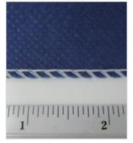
Figure 3. Normal 3-thread seam
