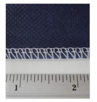
Figure 2. Stronger 4-thread overlocked seam
